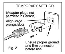
adapter, where local codes permit, a TEMPORARY CONNECTION may be made to a properly grounded two-prong wall receptacle by the use of a UL listed adapter (Fig. 2) which is available at most local hardware stores.
